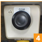
4 "Clear" button for jams & replacing bottom tape roll (Opposite Side of Machine)
